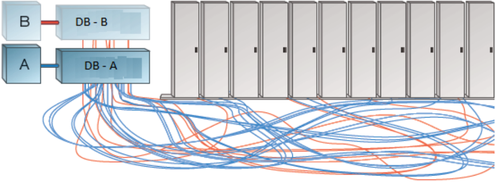
Fig. 3. Conventional power supply to data centre
